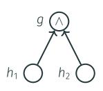
$$(h_1 \vee \overline{g})(h_2 \vee \overline{g})(\overline{h}_1 \vee \overline{h}_2 \vee g)$$
